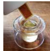
Step 5 Test system water
