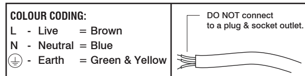
WIRING DIAGRAM - MAINS SUPPLY
