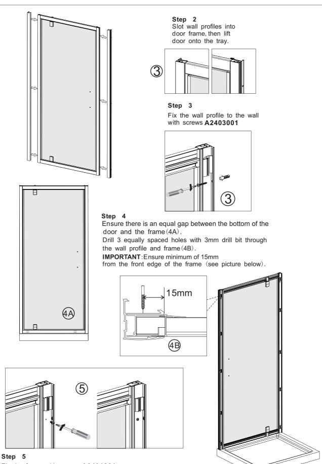
Fix the frame with screws A2401201
