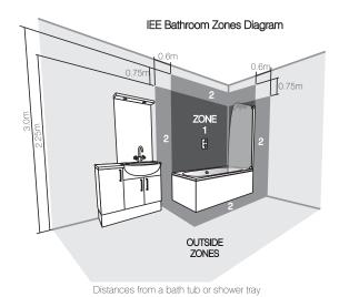
Bathroom fittings are subject to the appropriate zones in accordance with IEE Regulations. This product is **only** suitable for permanent indoor installation in Zone 2 and outside zones. (See above) This product is **not** suitable for installation in Zone 0 or 1, saunas, steam rooms or shower cubicles. Do **not** connect to a trailing plug and socket. Do **not** install onto surfaces that are either damp or electrically conductive.
