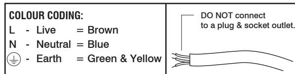
WIRING DIAGRAM - MAINS SUPPLY
