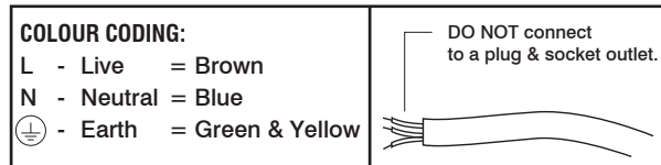
WIRING DIAGRAM - MAINS SUPPLY
