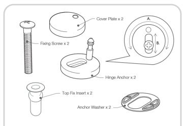
Maximum adjustment of the hinge anchor is achieved by rotating around the screw (adjustment A in the parts diagram above). Further fine adjustment of the hinge anchor can be achieved by sliding the screw in the hinge anchor (adjustment B).
