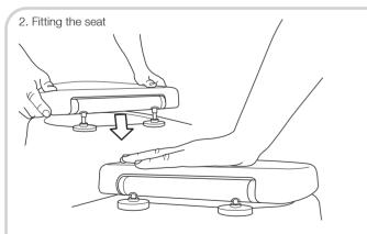
Align and insert the pins into the seat and firmly press down until you hear them 'click' into position. Adjust the hinge anchors to make sure the seat lines up with the edges of the toilet pan. When you are satisfied the seat is in the correct position, remove the seat from the hinge anchors (see step 3) and fully tighten the screw in the top fix insert (shown in step 1). Place the cover plates over the hinge anchors to cover the fixing screw.
