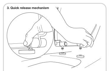
This toilet seat is designed for quick and easy removal when cleaning the toilet pan. To activate the quick release lift the lid and seat up. Press the buttons one by one and lift the seat up. To replace the seat align the sockets with the pins and firmly press down until you hear them click into position.
