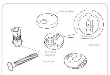
Maximum adjustment of the hinge anchor is achieved by rotating around the screw (adjustment A in the parts diagram above).
