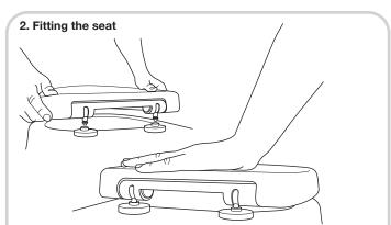
Align and insert the pins into the hinge achors and firmly press down until you hear them 'click' into position.
