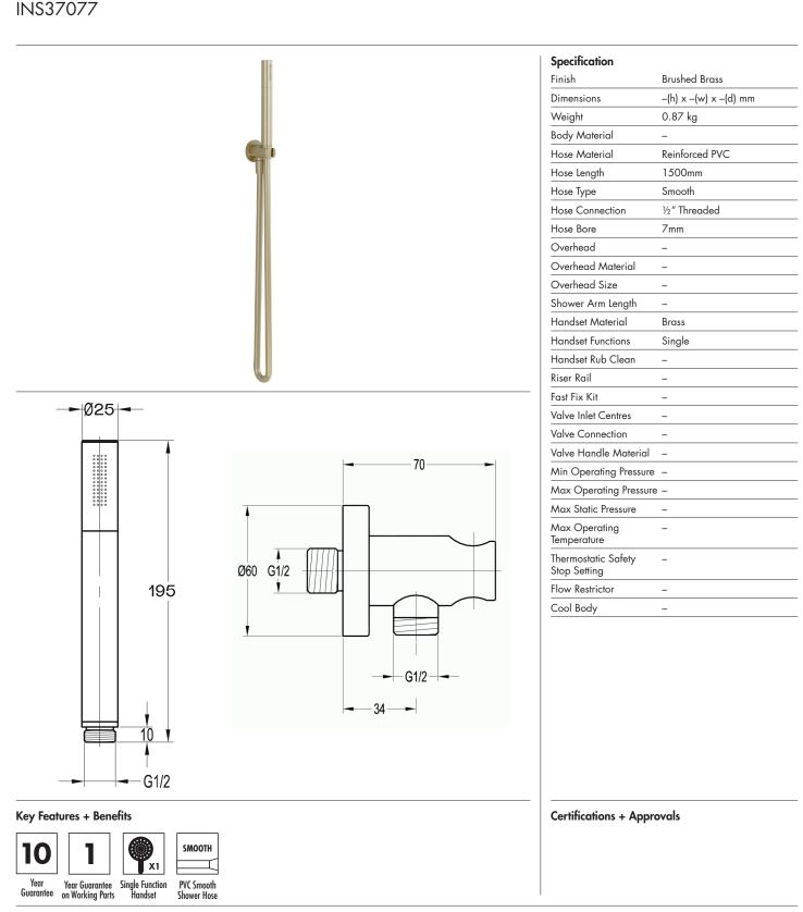
Keros Round Wall Outlet Elbow, Bracket, Smooth Hose + Round Pencil Brass Handset
