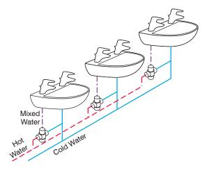
The Instinct range of thermostatic mixing valves **MUST** be installed in an accessible position to ensure that maintenance, commissioning and testing of the **Instinct Thermostatic Mixing Valves** can be undertaken easily.
