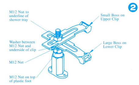
Position the tray in situation and level to the correct height as shown in diagram 4.
