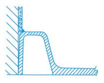
To prevent the possibility of water damage check all connections are water tight and that the tray is adequately sealed along the tiling line
