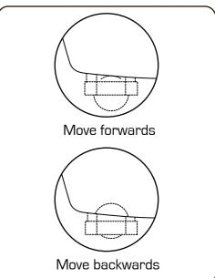
Please read carefully before attempting to fit the seat. If you are not the end user, please make sure the aftercare instructions are made available for the end user to read. Before fitting the seat to the pan it is essential that the hinges are adjusted correctly and the locking screws are firmly tightened. Failure to tighten these screws will result in the hinges working loose over a period of time.
