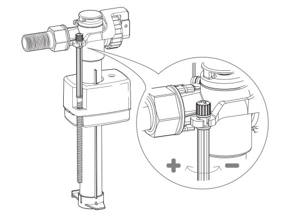
By adjusting the fill valve the water level can either be increased or decreased accordingly
