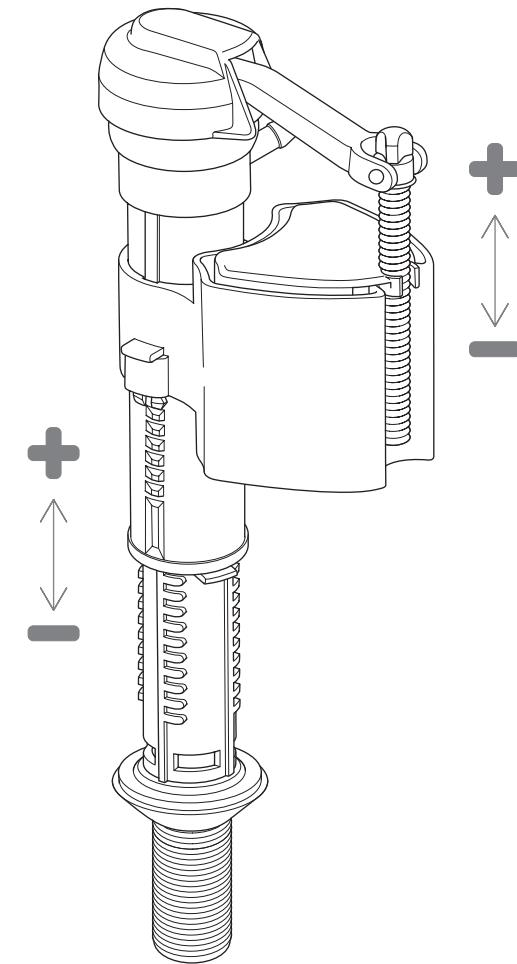
By adjusting the fill valve the water level can either be increased or decreased accordingly
