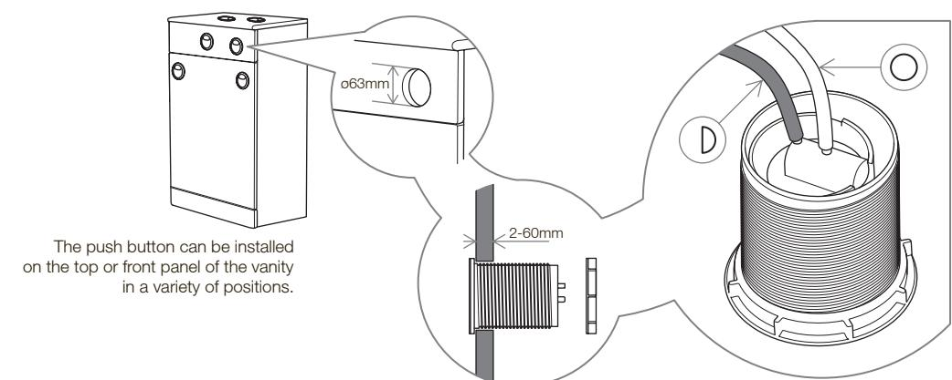
The push button can be installed on the top or front panel of the vanity in a variety of positions.
