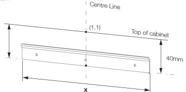
1.8 – Hang the cabinet on the wall bracket and check its level. Make sure the wall bracket has entered the slot and the cabinet is not resting on the edge of the wall bracket.
