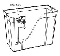
The fill valve is supplied at a height suitable for the cistern tank. Please ensure that all connections are fully tightened before progressing.
