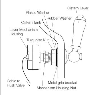
Rotate the handle up for a reduced flush. Rotate the handle down for full flush.
