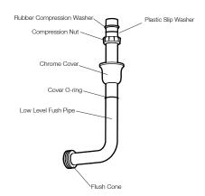
2. Put the parts labelled onto the flush pipe according to the diagram (Note that Flush Pipe, O-Ring and Chrome Cover are supplied separate to cistern in kit INST02006)
