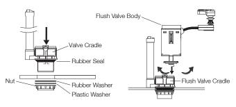
Ensure that the Flush Valve is assembled and fully tightened as shown.
