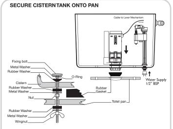
Mount the cistern to the WC pan as shown above. Ensure the gasket is firmly sealed around the flush channel. Once assembled the toilet can be positioned and installed in location. Before securing the pan to the floor, drill the holes in the wall for securing the cistern tank. After securing the pan to the floor, attach the tank to the wall using fixings suitable for the installation in hand (not supplied).
