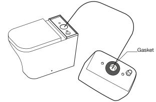
Insert the cistern fitting bolts arranging the components as shown in the diagram below.
