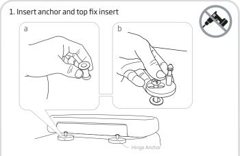
Place the rubber top-fix inserts into the fixing holes in the toilet pan (diagram a). Making sure that the rubber seals are installed, insert the screws within the hinge anchors, as shown in diagram b, and begin to tighten the screws until they are loosely secured, to allow for adjustment of the seat on the pan.
