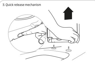
This toilet seat is designed for quick and easy removal when cleaning the toilet pan. To activate the quick release, raise the lid and seat. Press the button on the front of the hinge barrel and lift the seat up. To replace the seat align the hinge holes with the pins and firmly press down until you hear them click into position.
