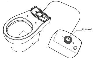
Insert the cistern fitting bolts arranging the components as shown in the diagram below.
