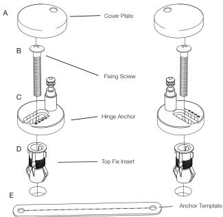
Note - alternative nuts and washers are supplied if you wish to secure the seat from underneath the deck of the toilet pan. If so dispose of the top fix inserts and tighten with the fixing key supplied.
