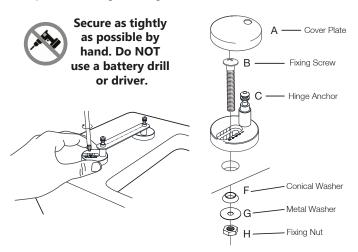
3 Remeasure the distance, making sure the 438mm dimension is met and remove the template and add the cover cap.
