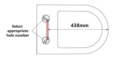
Once the 438mm dimension shown above is met and the template is parallel to the back edge, insert the bolts then tighten using a screw driver.
