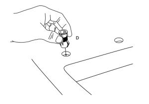
2 Place the template over the anchor pins, selecting the appropriate hole numbers (on the anchors) so that the 438mm dimension from the front of the pan to the centre line of the template is met.
