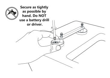
4 Remeasure the distance, making sure the 438mm dimension is met and remove the template and add the cover cap.
