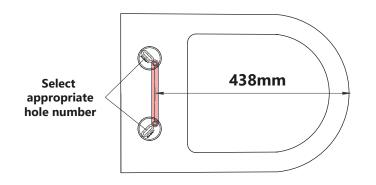
2 Once the 438mm dimension shown above is met and the template is parallel to the back edge, insert the bolts and tighten the underfix components, then tighten using a screw driver.
