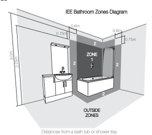
Bathroom fittings are subject to the appropriate zones in accordance with IEE Regulations. This product is only suitable for permanent indoor installation in Zone 2 and outside zones. (See above) This product is not suitable for installation in Zone 0 or 1, saunas, steam rooms or shower cubicles. Do not connect to a trailing plug and socket. Do not install onto surfaces that are either damp or electrically conductive.
