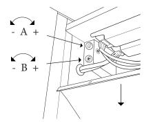
4.2 – After all cabinet hanger adjustments are complete, close the electrical compartment and screw shut using provided screws.
