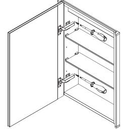
4.3 – Check the cabinet is flush and securely fitted to the wall.
