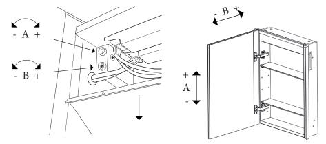
2.9 – When the cabinet is level, mark the hole on the lower section of the cabinet backboard (2.9). Take the cabinet off the wall.
