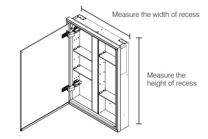
1.2 - Mark out the recess on the wall. Special attention must be taken to ensure there is nothing within the desired recessed space.
