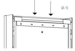
2.2 – When the cabinet is level, mark the hole on the lower section of the cabinet backboard. Take the cabinet off the wall.
