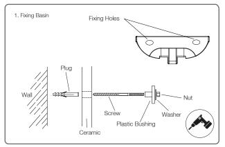
Ensure the wall is strong enough to support the basin and semi pedestal. Hold the basin up to test and ensure optimum height (recomended 800-850mm from tap deck to floor). Make sure the semi pedestal will cover the pipework when placed over and then mark out and drill the holes for the basin. The plugs and screws can then be inserted and tightened with a spanner.
