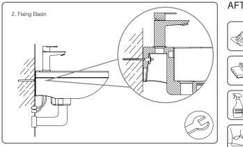
Place the basin over the screws and use the plastic bushing and nut to tighten into place. Tighten evenly by hand and finish off with a spanner.
