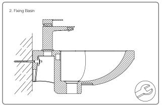
The tap and waste can be installed on the basin before securing to the wall using Plumber's Mait. Place the basin over the screws and use the plastic bushing and nut to tighten into place. Tighten evenly by hand, not tightening all the way to be able to lift the basin and fit the pedestal underneath.
