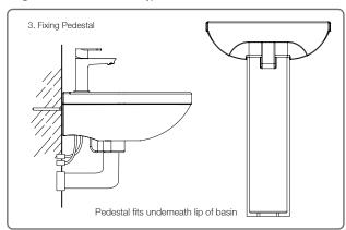
Attach the hot and cold feeds for the tap and the waste to the pipework.
