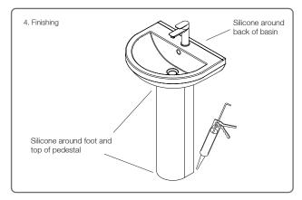
To finish the installation, silicone sealent with a gun can be used to go along the back of the basin, between the basin and pedestal and pedestal and floor.
