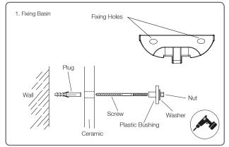
Ensure the wall is strong enough to support the basin. Make sure the pedestal will cover the pipework when placed over with the basin fitted. Mark out with basin in place and then drill the holes for the basin. The plugs and screws can then be inserted. The fixing set for washbasin is not included and different fixings are available for the wall type.
