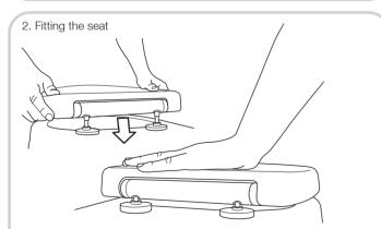
Align and insert the pins into the seat and firmly press down until you hear them 'click' into position. Adjust the hinge anchors to make sure the seat lines up with the edges of the toilet pan. When you are satisfied the seat is in the correct position, remove the seat from the hinge anchors (see step 3) and fully tighten the screw in the top fix insert (shown in step 1). Place the cover plates over the hinge anchors to cover the fixing screw.
