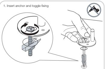
Insert the screws, toggle fixing and nut into the seat fixing holes of the toilet pan as shown. Lift the hinge anchor back up to engage the toggle fixing on the underside of the pan. Begin to tighten the screws until they are loosely secured, to allow for adjustment of the seat on the pan.
