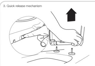
This toilet seat is designed for quick and easy removal when cleaning the toilet pan. To activate the quick release, raise the lid and seat. Press the button on the front of the hinge barrel and lift the seat up. To replace the seat align the hinge holes with the pins and firmly press down until you hear them click into position.
