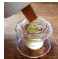
Step 5 Test system water
